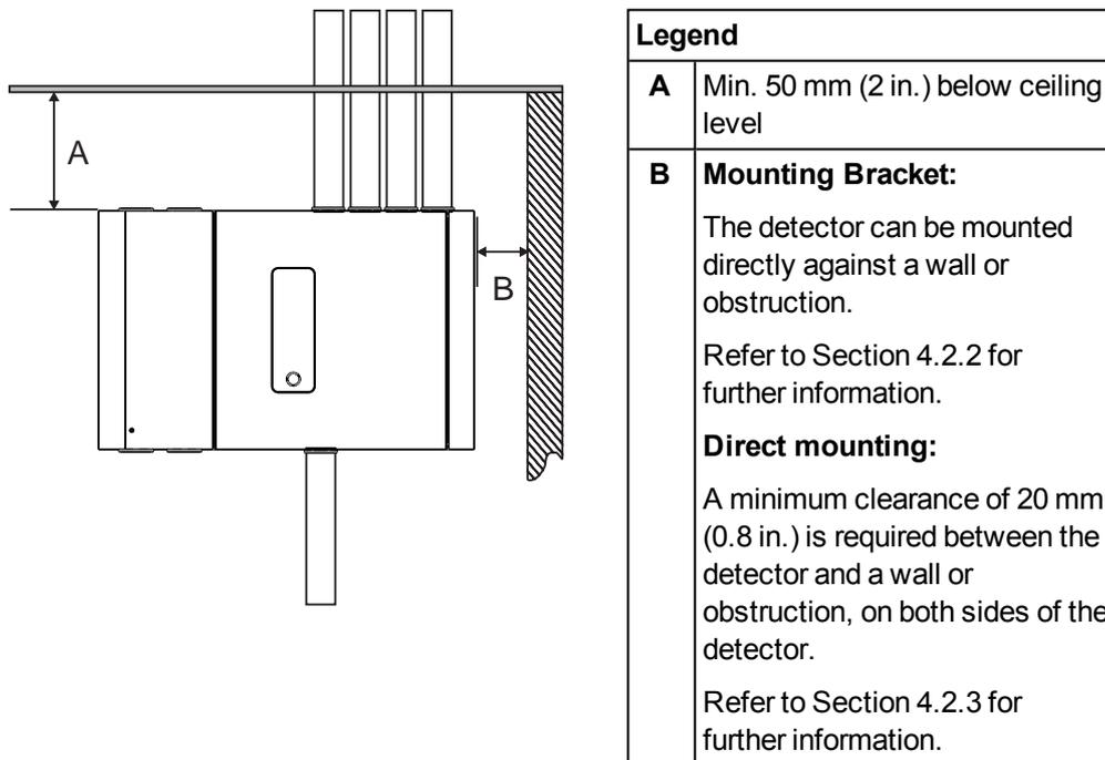
Figure 4-4: Mounting location
