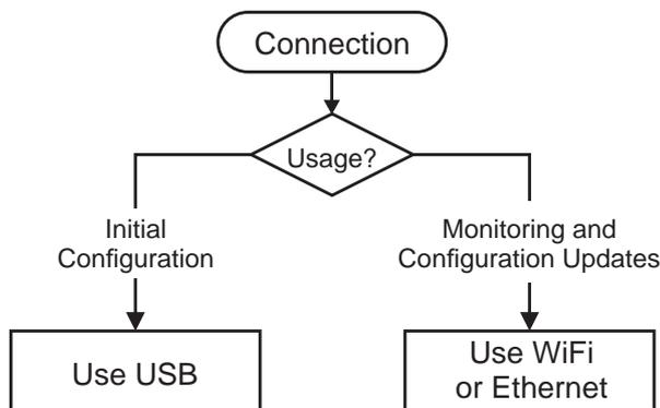
Figure 2-3: Connection Method
