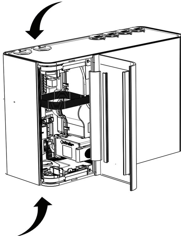
Figure 4-32: Cabling Inlets
