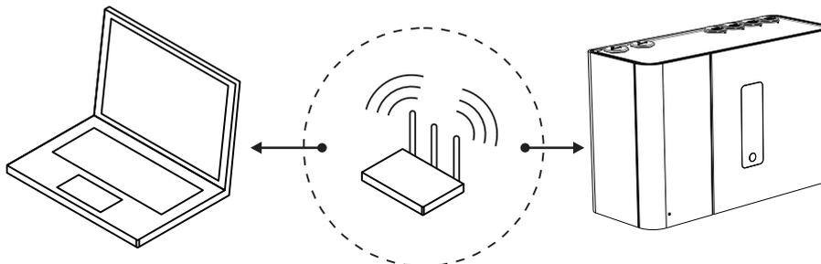
Figure 5-10: Connecting to a detector via WiFi using a router
