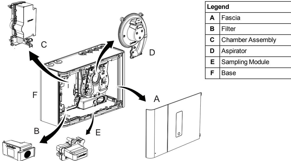
Figure 2-1: Detector components
