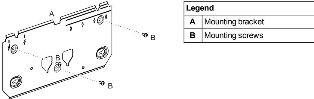
Figure 4-20: Mounting Bracket
