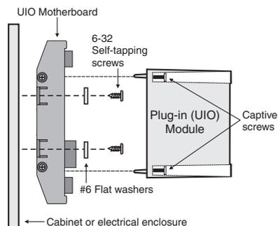
GE Security recommends that this module be installed according to latest recognized edition of national and local fire alarm codes.
