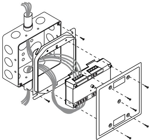
**SIGA-MCC1 and SIGA-MCC2:** mount the UIO motherboard inside a suitable GE Security enclosure with screws and washers provided. Plug the SIGA-MCC1 or SIGA-MCC2 into any available position on the motherboard and secure the module to the motherboard with the captive screws. Wiring connections are made to the terminals on the motherboard (see wiring diagram). UIO motherboard terminals are suited for #12 to #18 AWG (2.5 mm<sup>2</sup> to 0.75 mm<sup>2</sup>) wire size.
