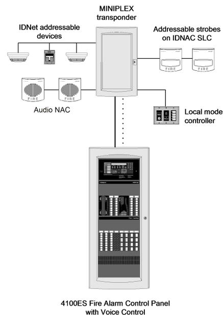
Figure 1: Typical 4100ES MINIPLEX System One-Line Drawing
