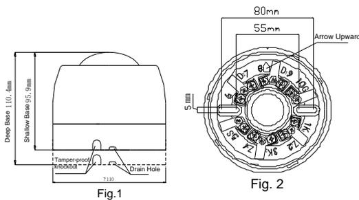
Z1 (2), Z2 (4): Loop of the control panel, polarity-insensitive.
