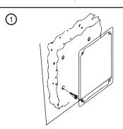
First drill the installation hole on the wall with a pistol, then put the installation plastic particles into the hole, and then align the sea ling rubber ring of the raised base with the hole.
