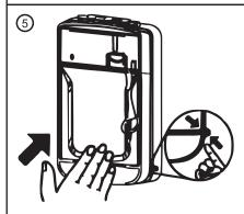
After the fixing test is completed, finally align the ear of the shell with the buckle of the base and press the buckle to complete the installation.
