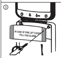
Then align the bottom surface of the main body with the holes of the fixed heightened base and tighten and fix it with the standard short screws.
