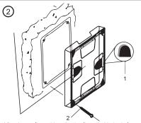
After the sealing rubber ring is aligned with the hole position, first clamp the standard black sponge to the mouth of the raised seat, then align the raised base with the screw hole, and then tighten it with the extension screw until it is firmly fixed.
