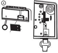
Install the battery in the internal alarm, and then use the pull cord to pull the test.
