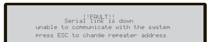
**Figure 55** Display "the repeater link is down".
