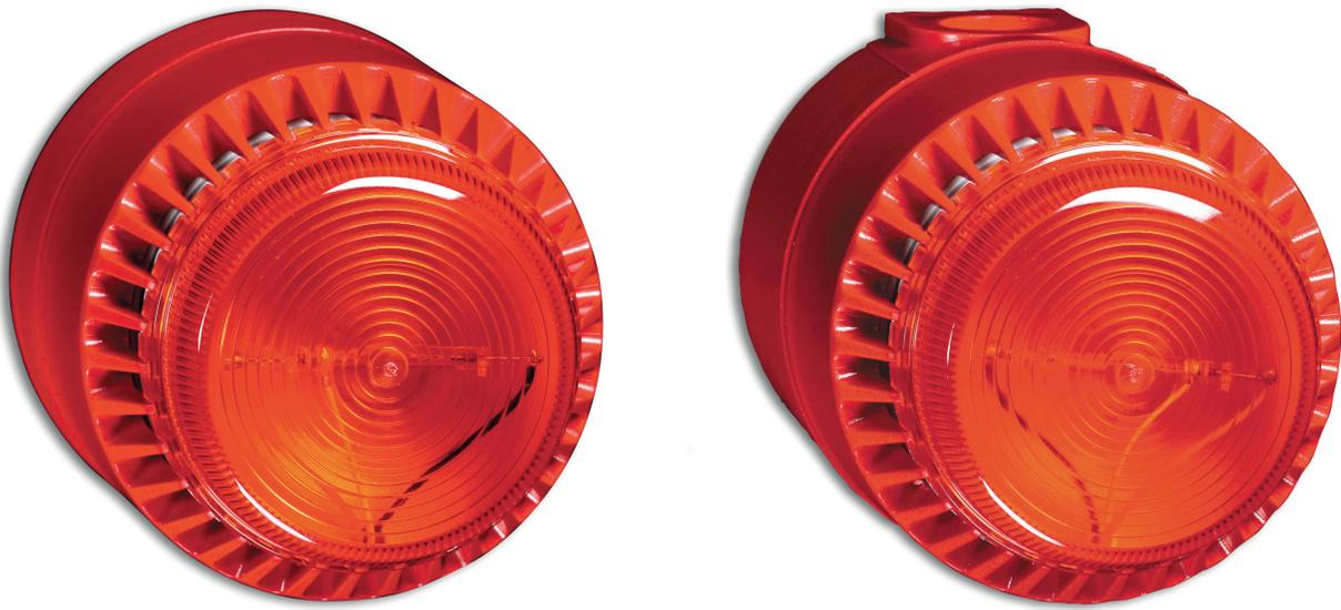
The Xenon sounder indicator is an audible and visual device which requires one single installation point. This greatly reduces installation costs and is less obtrusive than two separate devices. Versions are available with the sounder and beacon linked, or with separate terminals for independent operation.
