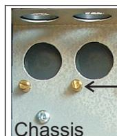
\* The cable screens must be connected to an **earth terminal** on the chassis or in the metal box.
