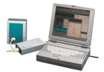
The PC - Link High Level Interface (PC - Link HLI) connects a PC and VESDA system. Each PC - Link HLI includes two cables (It does not include a PC):
